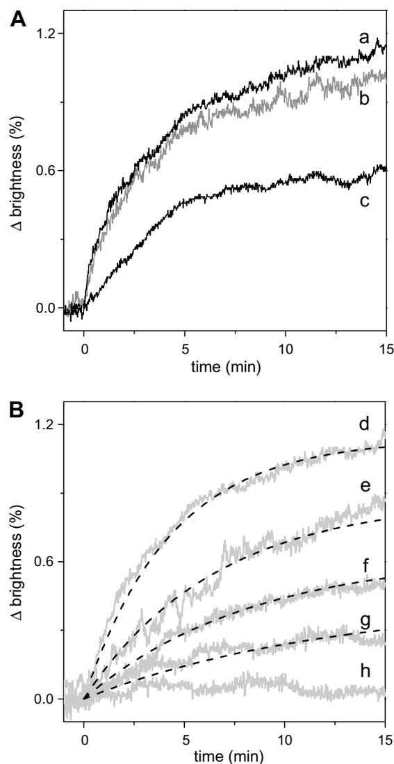
**Fig. 6.** Dependence of the transient scattering signal corresponding to the BSA antibody–antigen binding on the chosen reference and the concentration of a BSA in analyte solution. (A) Fixed [aBSA] = 28 nM with varying reference: (a) glycine; (b) IgG; (c) fibrinogen. (B) Glycine reference with varying [aBSA]: (d) 28 nM; (e) 18 nM; (f) 14 nM; (g) 9 nM; (h) control buffer injection. Dashed curves are simulations based on  $k_a = 1.3 \times 10^5 \text{ M}^{-1} \text{ s}^{-1}$ .
