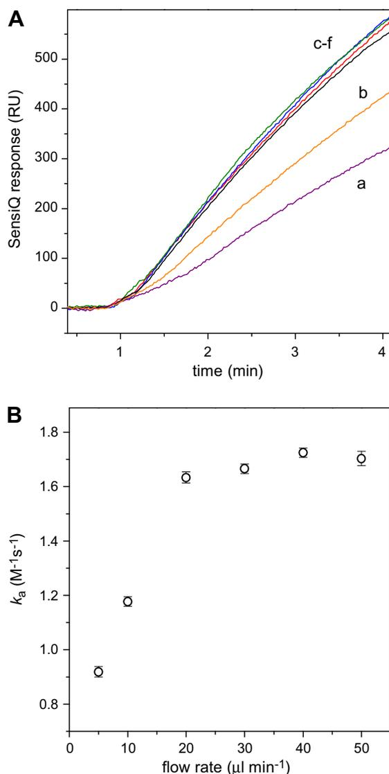
**Fig. 5.** Effect of the analyte flow rate used in the SensiQ-based experiments on the observed BSA antibody–antigen association rate. (A) Transient response curves corresponding to 5- $\mu l/\text{min}$  (a), 10- $\mu l/\text{min}$  (b), 20- $\mu l/\text{min}$  (c), 30- $\mu l/\text{min}$  (d), 40- $\mu l/\text{min}$  (e), and 50- $\mu l/\text{min}$  (f) flow rates of approximately 14 nM anti-BSA analyte solution. (B) Association rate constants derived from the curves shown in panel A.
