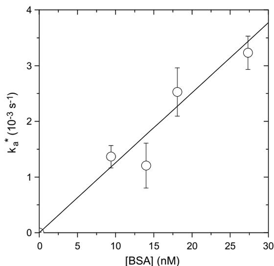
**Fig. 8.** Pseudo-first-order rate constants for BSA antibody–antigen binding derived from light scattering array sensor data. The slope from the linear fit corresponds to the second-order rate constant  $k_a = (1.3 \pm 0.3) \times 10^5 \text{ M}^{-1} \text{ s}^{-1}$ .
