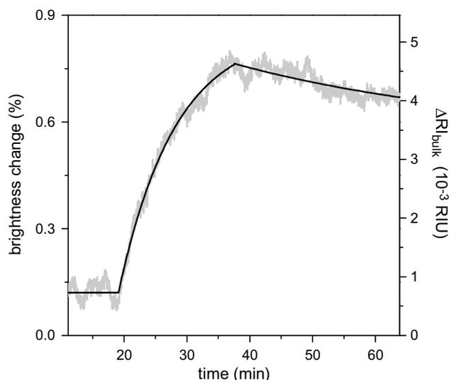
**Fig. 7.** Transient scattering signal observed on sensor array exposure to the 9.5-nM BSA antiserum solution using a glycine reference spot. Solid black curves correspond to the best fit curves from Eq. (4):  $k_a = (1.4 \pm 0.2) \times 10^5 \text{ M}^{-1} \text{ s}^{-1}$  and  $k_d = (4 \pm 2) \times 10^{-4} \text{ s}^{-1}$ .
