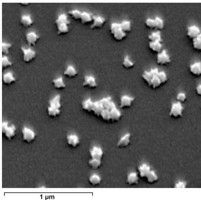
Fig. 2. SEM image of the nanoparticles grown from gold seed particles deposited on silica substrate. Coverage =  $14 \pm 2\%$ ; size =  $130 \pm 6$  nm.
