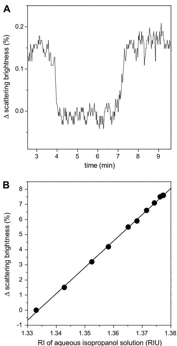
Fig. 4. (A) Sensitivity to the change of the bulk  $RI$  on switch of the analyte solution from 1% aqueous isopropanol to water. Estimated  $RIS = 1.5 \pm 10^{-4}$  RIU. (B) Linearity of the light scattering response to the change in the bulk  $RI$  of the analyte solution.  $r^2 = 0.9992$ ;  $\chi^2 = 5.796 \times 10^{-7}$ .
