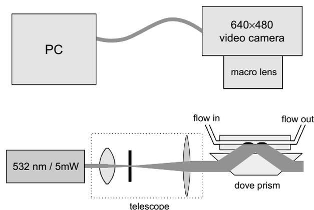
Fig. 1. Schematic diagram of the sensor array reader.
