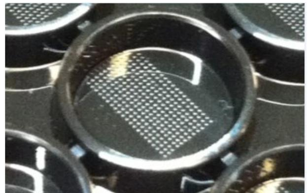
Fig. 3 ProxiPlate-96 well spot printing.
