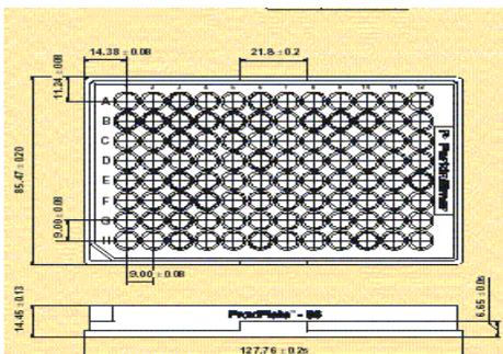
Fig. 1 ProxiPlate-96 (Perkin Elmer, Product No 6006270)
